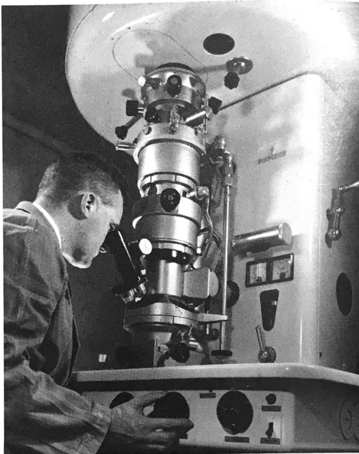
THE ELECTRON MICROSCOPE, with magnifications as high as 100,000, has made it possible for the scientist to explore the ultra-fine structure of cells and organisms. Its immense power of detecting the most minute detail has enabled research workers to determine certain physical differences between normal and cancer cells.
