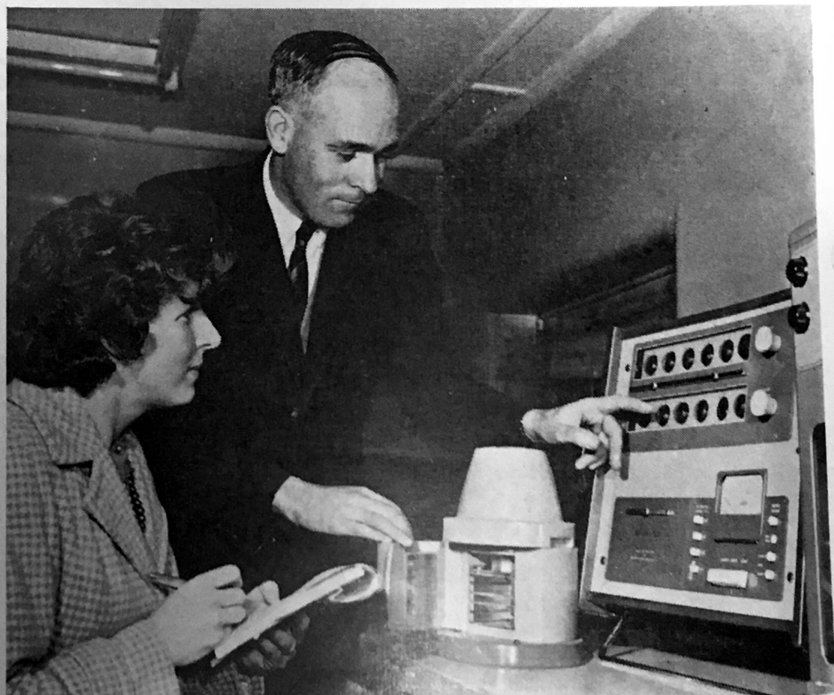
THE EQUIPMENT USED TO MEASURE RADIOACTIVITY IN RAT LIVER TISSUE following administration of a radioactive substance, is demonstrated by Dr. Hughes to a student reporter. The tissue is placed in the lead "castle" (centre) which shields background radiation from the specimen, while the Geiger counter (right) records the amount of radioactivity present.
